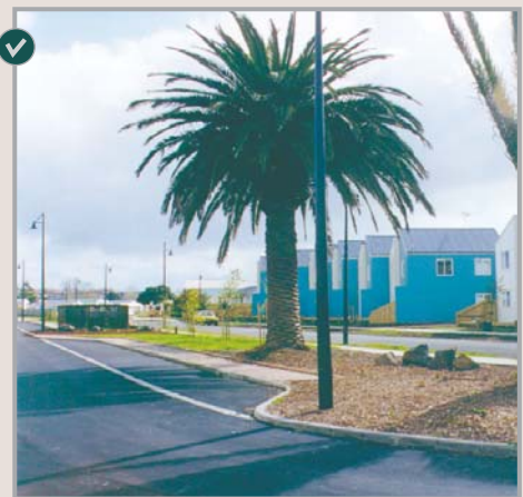
Restricting parking to one side of the road, and kerb shaping aids safety and visual amenity.
