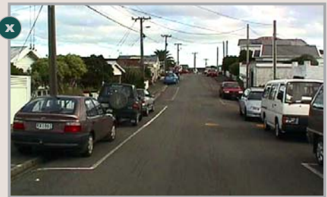
Restricting parking to one side of the road, and kerb shaping aids safety and visual amenity.
